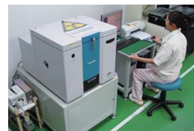
Parts inspection using a fluorescent/X-ray analyzer.
